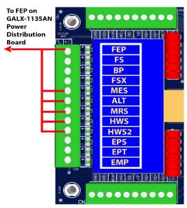
Figure 1: Typical I/O Expansion Board Fire I/O Board
