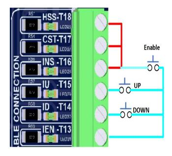
Figure 2: GALX-1121 Main I/O Board With Run Bug. See Figure 3 For Run Bug Stop Switch.
