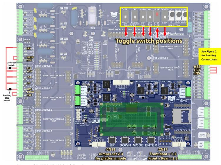
Figure 3: GALX-1121AN Main I/O Board
